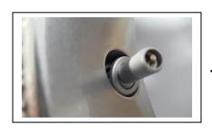
CAREFULLY INSTALL THE WASHER AND ENSURE IT IS SEATED CORRECTLY
