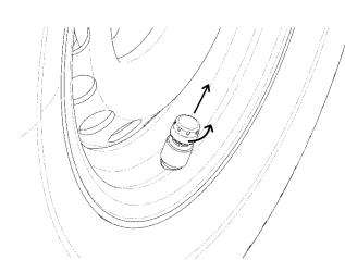
WHILST HOLDING THE MONITOR 1.5M AWAY FROM TYRE, REMOVE SENSOR FROM TYRE VALVE STEM. MONITOR SHOULD ALARM. REPLACE SENSOR TO CANCEL ALARM.
