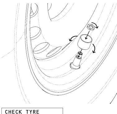
NOTE: WHEN THE DUST SHIELD IS FITTED FOLD IT BACK ON ITSELF. THIS MAKES IT EASIER TO FIT LOCK NUT AND SENSOR.
