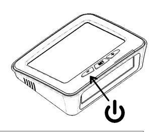
PRESS AND *HOLD* "-" BUTTON FOR 4-5 SECS TO TURN MONITOR ON
