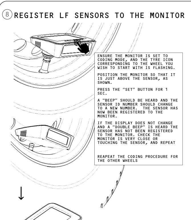
PRESS AND *HOLD* THE "SET" BUTTON FOR 4-5 SECS TO REGISTER THE SENSOR ID SETTINGS
