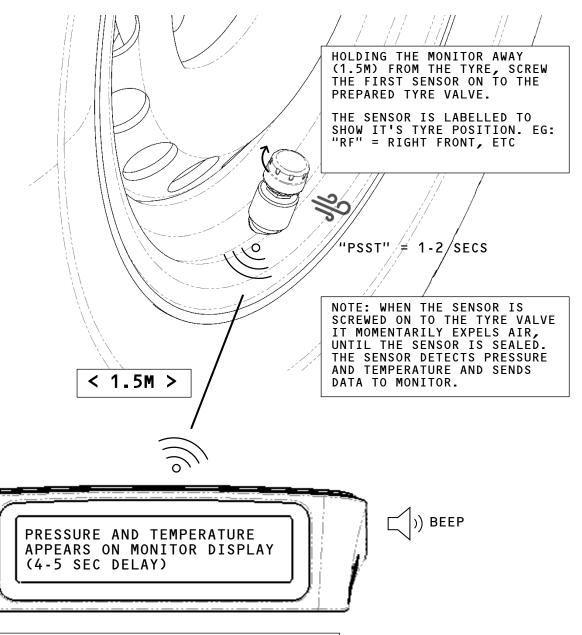
NOTE: TCSO SENSORS ARE SUPPLIED PRE-REGISTERED TO THE MONITOR. EACH SENSOR IS LABELLED TO SHOW THE WHEEL/TYRE IT IS REGISTERED TO. FOR EXAMPLE, A SENSOR LABELLED "RF" SHOULD BE FITTED TO THE RIGHT FRONT WHEEL (THE RIGHT HAND SIDE OF THE CAR IS DEFINED AS THE SIDE ON THE DRIVER'S RIGHT WHEN SEATED AND FACING FORWARD)
