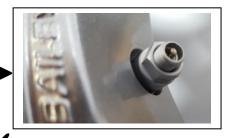
ATTACH THE THREADED COLLAR WITH HEXAGON UPPERMOST, AS SHOWN
