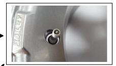
ENSURE THE SENSOR RUBBER SEAL AND VALVE STEM ARE SEATED SQUARE
