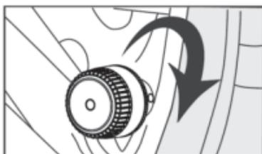
The monitor beeps and stores the tyre position with that sensor ID. If it does not register within a few seconds, unscrew the sensor and try again.
